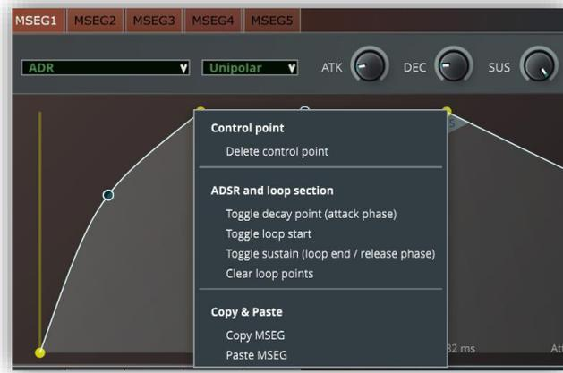
You can drag the unfilled circles up and down to change the steepness (curviness) of the envelope segment between two points.
