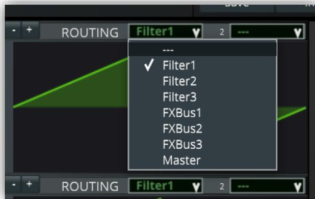
You can select up to two different audio routing targets per generator. With this you can split the signal and process both part individually.
