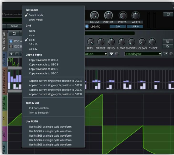
In the context menu you can choose to display a grid for selection or the draw mode. Selection and drawing will be snapped to the grid then.
