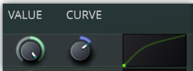
Once a parameter is modulated (either by drag & drop or by manual assignment) it will be marked with yellow color to indicate the modulation behavior. The modulation center and amount are indicated with the yellow range. You can change this range either in the modulation matrix or by dragging with a right mouse-click up and down. The center of the modulation controlled by the parameter value itself.
