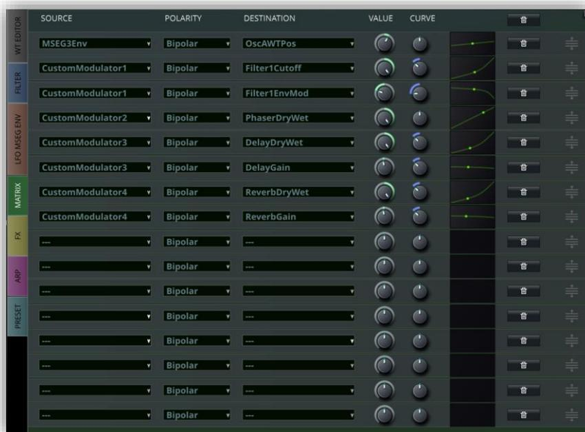
The mechanism behind the modulation matrix is to define an input source (e.g. LFOs, envelopes ...) that modulates a modulation destination with a defined intensity and behavior controlled by the modulation matrix value. With the 16 modulation matrix slots, the positive and negative modulation curves and the 11 input sources and the >200 destinations Vaporizer2 supports more than 100.000 possible different modulation combinations.
