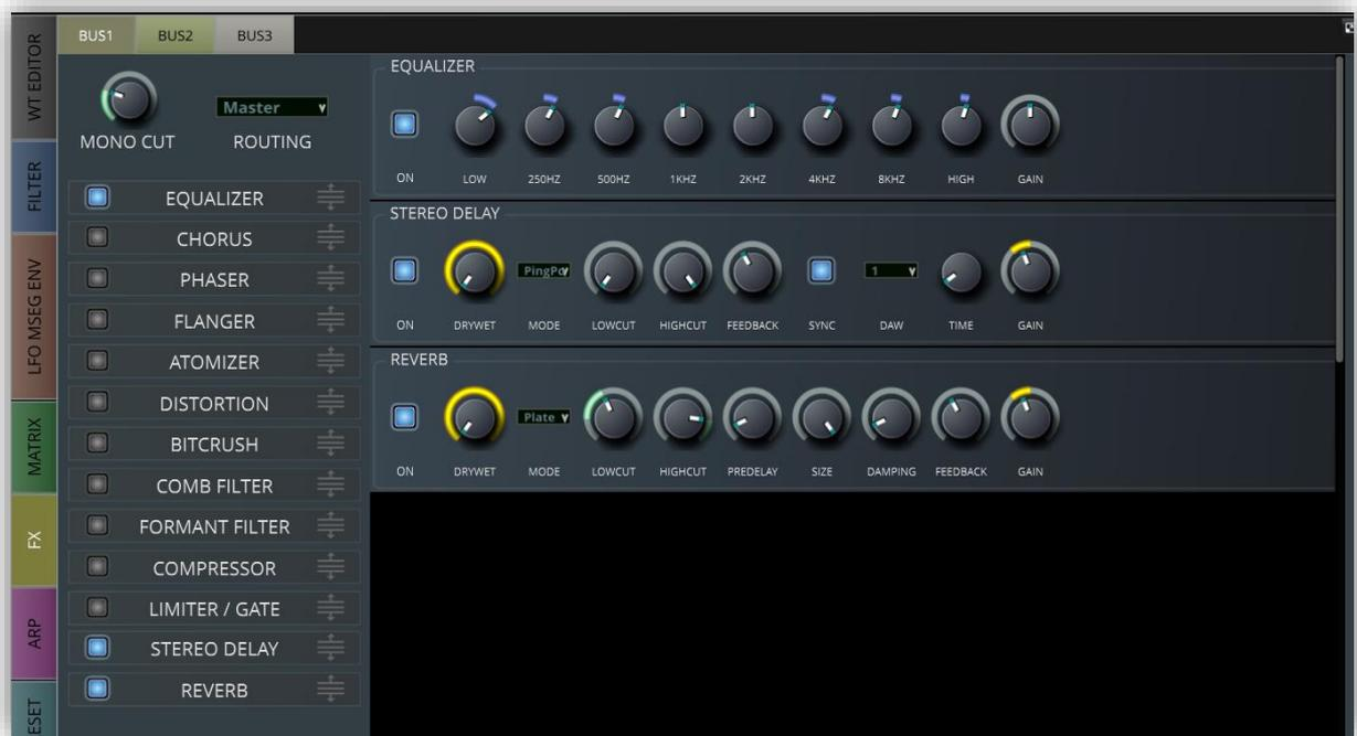
All effects can be switched on / off individually and can be mixed in and out by using a dry / wet parameter.
