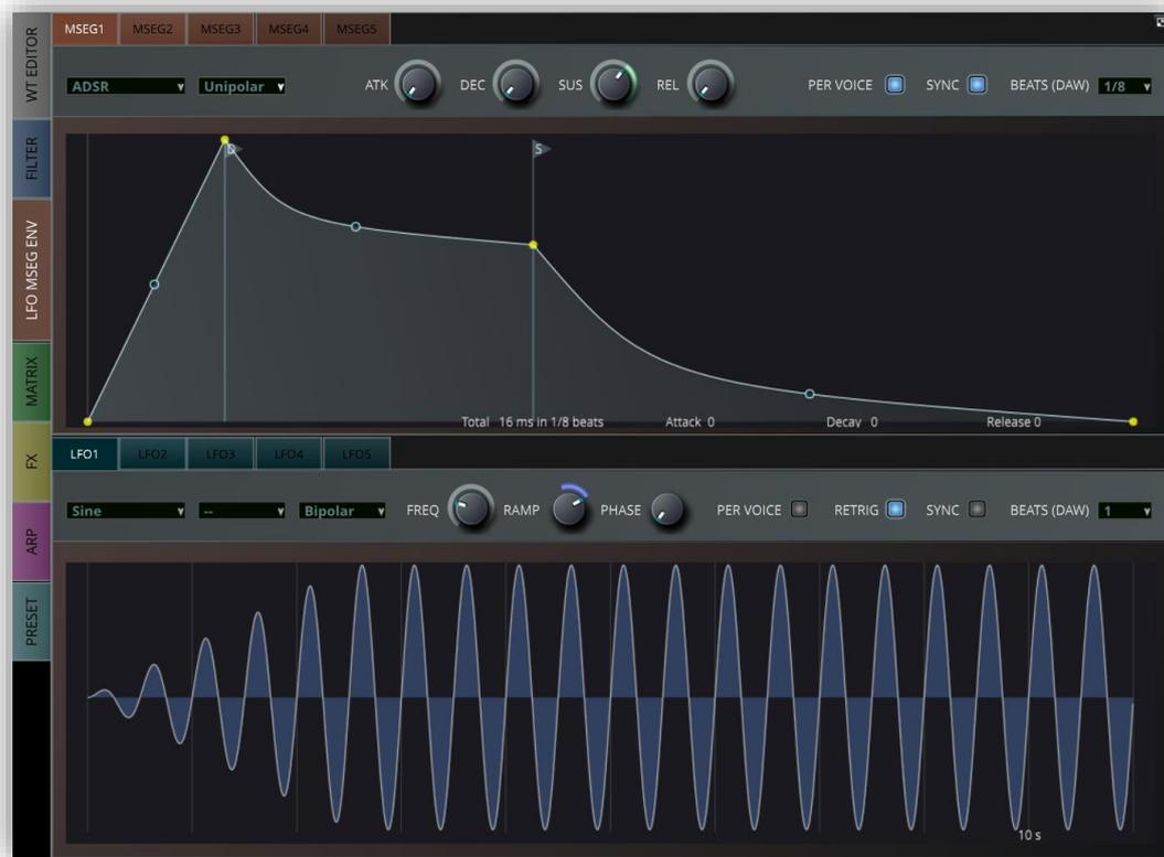
You can preselect a common shape from the drop-down box. But you can also create a completely new envelope shape. For this just right-click on the envelope and select from the context menu. You can add or delete control points here. You can also mark a control point as a
