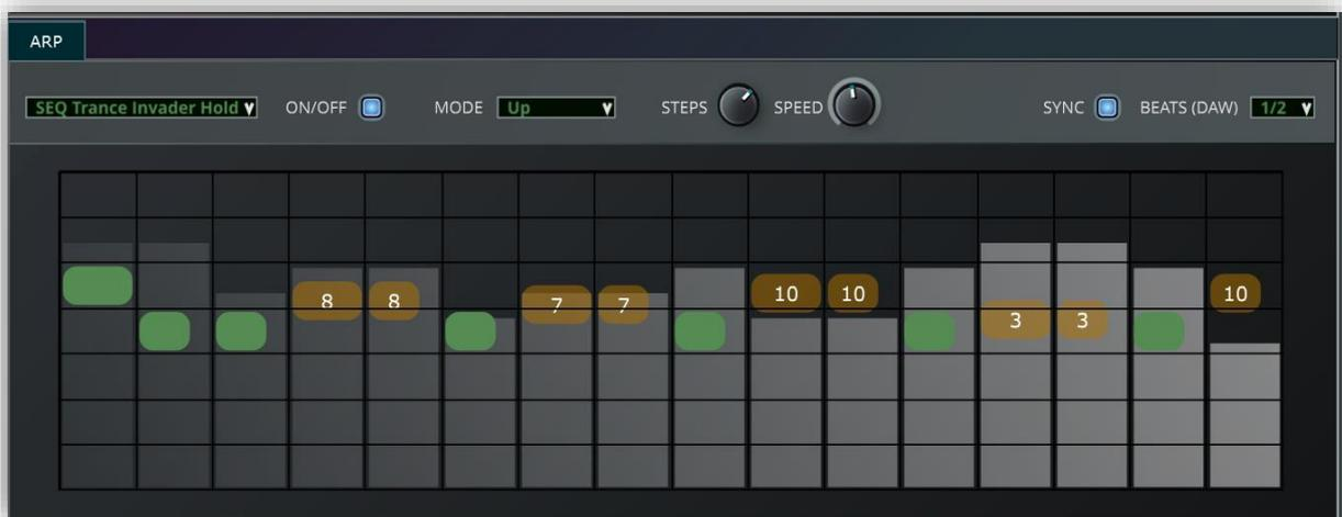
The arpeggiator can be synced to the DAW time code or can be free running. When free-running (SYNC switched off) the speed is derived from the SPEED setting. When synced to DAW the DAW's beats per minute setting controls the speed by calculation fractions of whole notes defined by the BEATS(DAW) setting. E.g. quarter notes are defined by a value of "4". E.g. triples can be set up with a value of "3".
