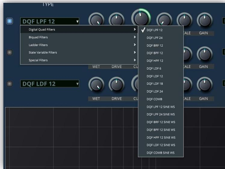
All filters support a WET setting (which controls the dry / wet rate of the signal going in and out of the filter), a filter DRIVE (i.e. a pre-gain amplification / attenuation of the signal going in the filter), a CUTOFF frequency and a resonance (RESO) level. Note that for some filter effects a certain drive level is helpful to achieve the desired effect.
