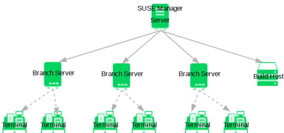
Branch servers should be physically located close to point-of-service terminals, such as in an individual store or branch office. We recommend you have a fast network connection between the branch server and its terminals. Branch servers provide services for PXE boot, and act as an image cache, Salt broker, and proxy for software components (RPM packages). The branch server can also manage local networking, and provide DHCP and DNS services.
