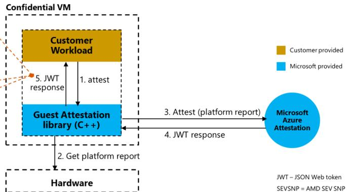
To perform attestation, the customer workload must integrate with the attestation library and run inside a confidential VM. Upon making a request to the attestation library, the customer workload can parse the response to determine if the VM is running on a desired hardware platform, and/or secure boot setting to continue to fully setup the sensitive workload.
