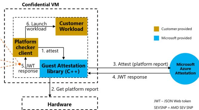
To perform attestation, a client program (called Platform checker client in diagram) must integrate with the attestation library and run inside a confidential VM. Upon making a request to the attestation library, the client program can parse the response to determine if the VM is running on a desired hardware platform, and/or secure boot setting to launch the sensitive workload.
