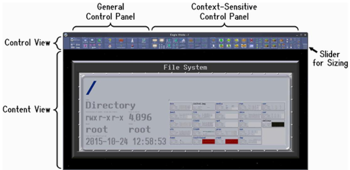
There is a slider for sizing the control view. You can drag it up and down with the left mouse button. A double click on it minimizes or unminimizes the control view.
