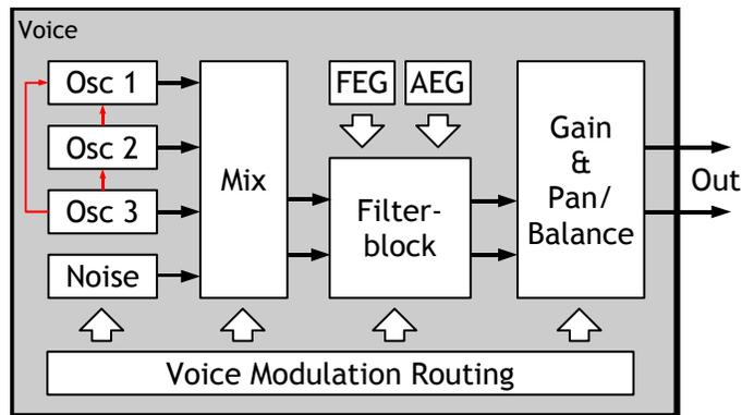
Illustration 17: Block diagram of a synthesizer voice
