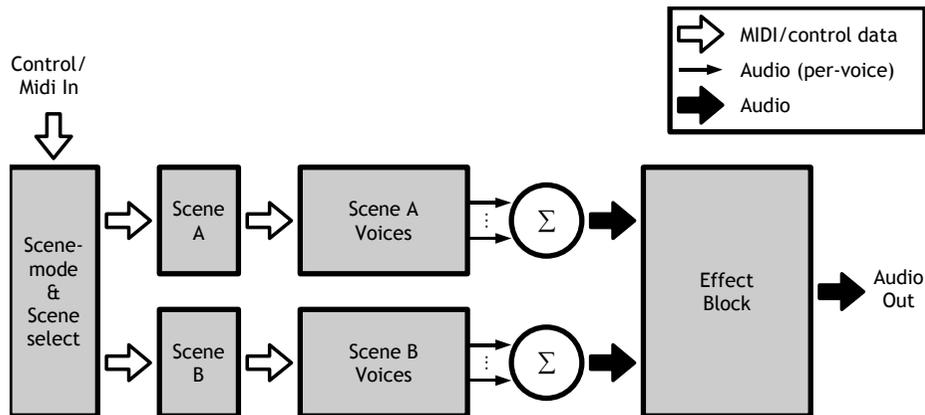
Illustration 16: Block diagram of the synthesizer engine.
